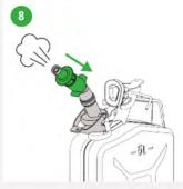
Before filling the fuelpress the tip of the spout to even out the fuel pressure in the fuel can.
