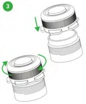
Place the cap back on the neck of the fuel can. Close the fuel can shut by screwing the cap clockwise.
