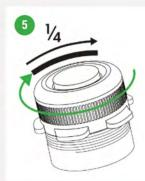
Screw the cap until you feel resistence. Then turn the cap an additional 1/4 of a turn.
