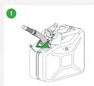
Push the lever forward until the lid completely covers the neck opening.
