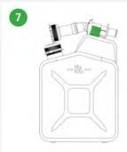
If the fuel can is equiupped with a fuel spout holder attach the spout for easier transportation.
