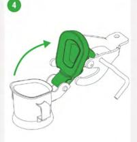
By pulling the lever, lift the lid up to open the neck opening.
