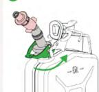
Move the arms of the lever into the cavities of the holder and push the lever of the spout down as far as it will go.
