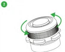
Open the fuel can by screwing the cap counterclockwise.
