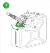
Move the arms of the lever into the cavities of the holder and push the lever of the spout down as far as it will go.
