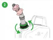
Unscrew the spout from the fuel can by turning it counterclockwise.
