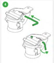
Insert the locking pin through the lever and rotate in 90degrees.
