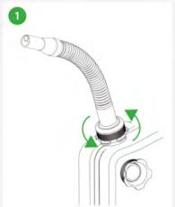
Unscrew the spout from the fuel can by turning it counterclockwise.
