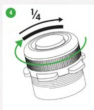
Screw the cap until you feel resistance. Then turn the cap an additional 1/4 of a turn. Do not tighten too much as it may be difficult to unscrew.
