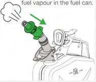
Pull back the level of the fuel spout to remove the product from the fuel can.
