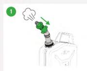
Press the tip of the spout to reduce the pressure of fuel vapour.
