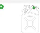
If the fuel can is equipped with a fuel spout holder, attach the spout for easier transportation.
