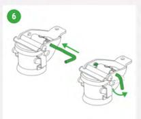
Insert the locking pin through the lever and rotate it 90 degrees.
