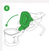
Push the lever forward until the lid completely covers the neck opening.
