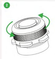
Open the fuel can by screwing the cap counterclockwise.
