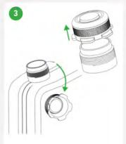
Place the removed cap on the fuel can with the help of the incorporated magnet.
