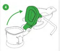
By pulling the lever, lift the lid up to openthe neck opening.
