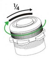
Screw the cap until you feel resistance. Then turn the cap an additional 1/4 of a turn. Do not tighten the cap too much, as it may be difficult to unscrew.
