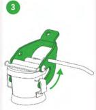
Lift the lever until the arms are fully released from the holder.
