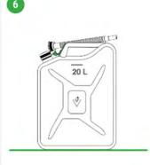
If the fuel can is equipped with a fuel spout holder, attach the spout to the holder for easier transportation.
