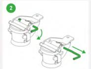
Turn the locking pin and pull it out of the level as far as it will go.
